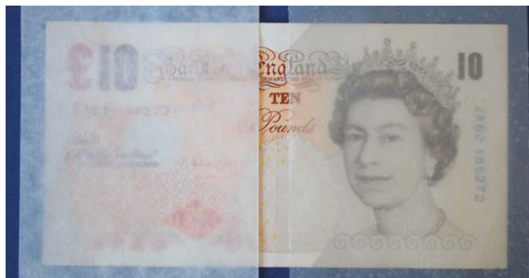
Figure 32: A comparison of the optical transparency of NFC and BC sheets. Left: BC sheet and right: NFC sheet.
