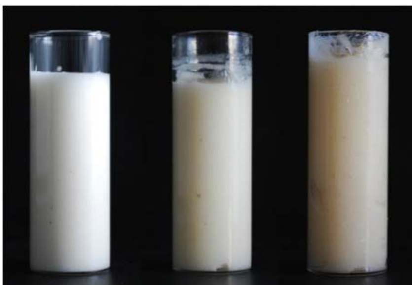
Figure 47: A photograph showing the gas-monomer liquid foam 5 min after mechanical frothing. Left: AESO 1 (0 wt.-% BC), middle: AESO 2 (0.5 wt.-% BC) and right: AESO 3 (1 wt.-% BC).
