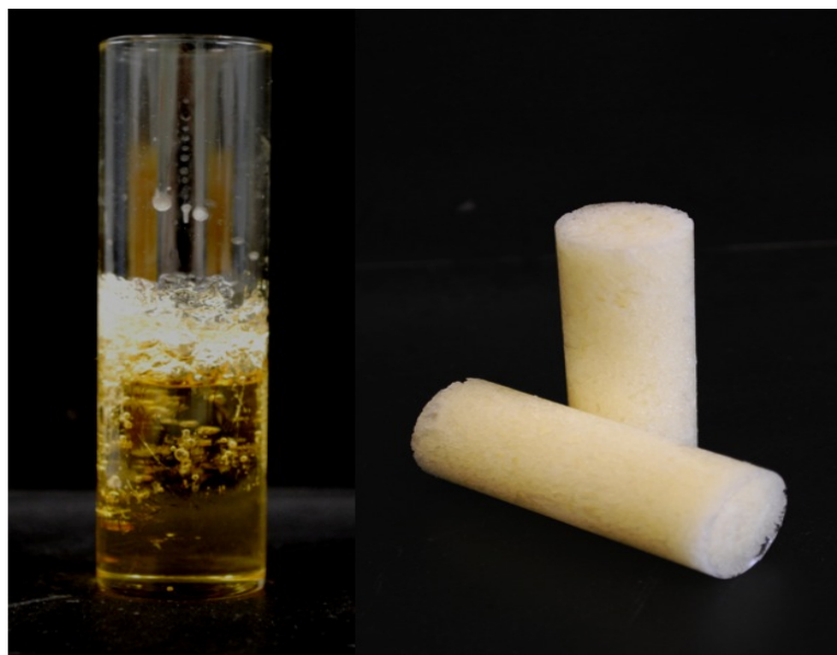
Figure 51: A comparison between non-mechanically frothed and air templated polyAESO. The photograph on the left shows polyAESO that was not mechanically frothed prior to its polymerisation and the image on the right shows the air templated polyAESO 1 (0 wt.-% BC).
