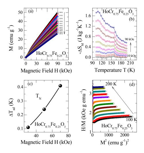
**Fig. 3:** (a) Isothermal magnetization (M) *vs.* magnetic field (H) curves in the temperature range 100 – 200 K (b) Temperature dependent magnetic entropy change  $-\Delta S_M$  in the field range 10 – 90 kOe (c) variation of adiabatic temperature change  $\Delta T_{ad}$  with magnetic field (d) Arrott plots corresponding to isothermal M *vs.* H curves for HoCr<sub>0.75</sub>Fe<sub>0.25</sub>O<sub>3</sub> compound.
