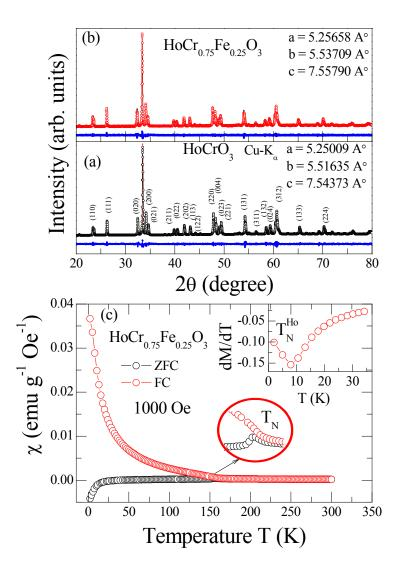
**Fig. 1:** Powder x-ray diffraction pattern recorded at room temperature pertinent to (a) HoCrO3 and (b) HoCr<sub>0.75</sub>Fe<sub>0.25</sub>O<sub>3</sub> compound. (c) Temperature dependence of susceptibility pertinent to HoCr<sub>0.75</sub>Fe<sub>0.25</sub>O<sub>3</sub> compound. Region pertinent to T<sub>N</sub> expanded for clarity. Inset of Fig. 1(c) shows the first derivative of field cooled (FC) M *vs.* T curve.
