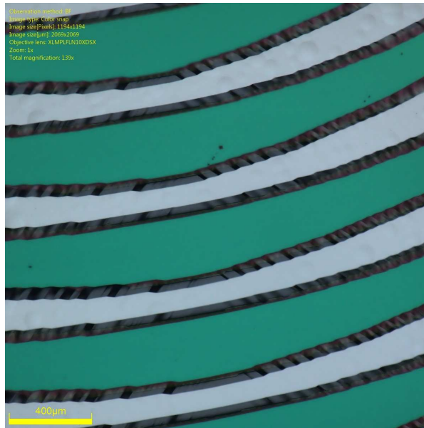
Figure 3.6: Circular spiral channel after etching in 25 wt% TMAH and 0.4% v/v Triton X-100
