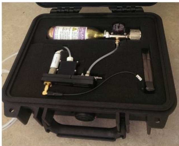
Figure 2.4: Photograph of a MEMS GC system components [4]
