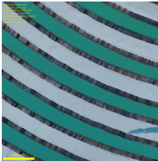
Figure 3.7: Circular spiral channel after etching in 25 wt% TMAH and 0.4% v/v Triton X-100 for 2 hours
