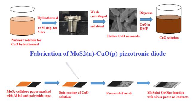
Figure 6.1: Schematic of the synthesis of  $MoS_2$  on cellulose paper, hollow CuO nanorods and fabrication of  $MoS_2$ -CuO piezotronic diode
