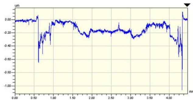
Figure 9.17 Wear Scar on the MTM Disc Tested with Salicylate + ZDDP (0.08 P wt%)
