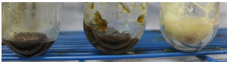
Figure 55: Dry pine specimens treated at 120°C for 15 h with [\text{C}_4\text{C}_1\text{im}][\text{Me}_2\text{PO}_4] (left), [\text{C}_4\text{C}_1\text{im}][\text{MeCO}_2] (middle) and [\text{C}_4\text{C}_1\text{im}]\text{Cl} (right). The specimen in the middle is a meshed pine chip.
