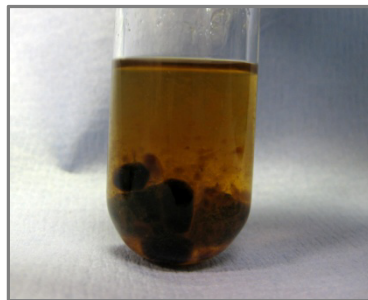
Figure 60: Pine chip regeneration in methanol after 18 h treatment with [\text{C}_4\text{C}_1\text{im}][\text{MeCO}_2] .
