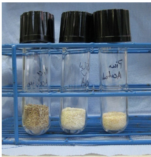
Figure 67: Capped glass tubes used for the ionic liquid pretreatment of ground lignocellulosic biomass: Miscanthus (left), willow (middle) and pine (right).
