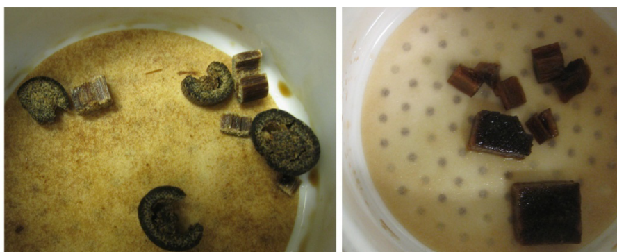
Figure 102: Miscanthus and willow chips pretreated with [\text{C}_4\text{C}_1\text{im}][\text{HSO}_4]_{80\%} at 120^\circ\text{C} for 22 h.
