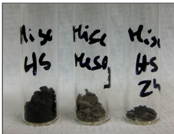
Figure 94: Miscanthus lignin precipitated from the pretreatment liquor. Left: after 22 h from [\text{C}_4\text{C}_1\text{im}][\text{HSO}_4]_{80\%} ; middle: after 22 h from [\text{C}_4\text{C}_1\text{im}][\text{MeSO}_3]_{80\%} ; right: after 2 h from [\text{C}_4\text{C}_1\text{im}][\text{HSO}_4]_{80\%} .
