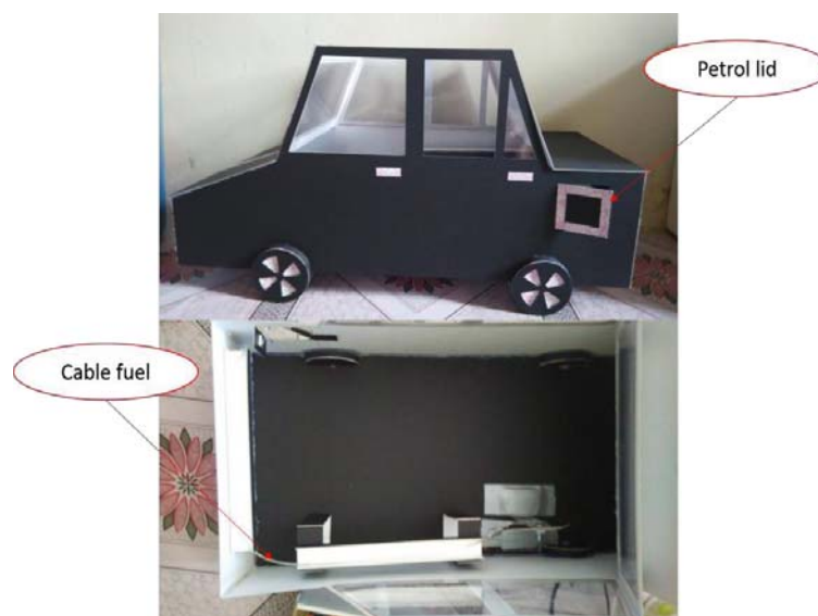
Figure 16. Model of car for operation of fuel lid and fuel cable.
