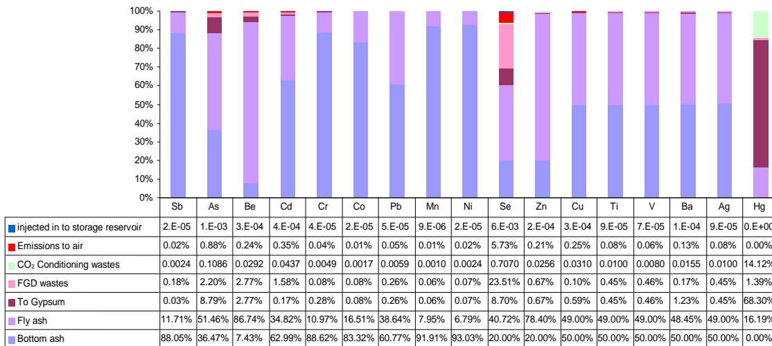
Figure 10.3: Partitioning of trace metals across the pollution control units in a 500 MW oxy-fuel combustion CO 2 capture power plant.
