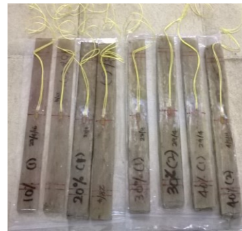
Figure 2. Composite samples with different fiber volume ratios.
