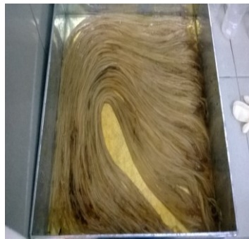
Figure 1. Fibers treated in NaOH solution.
