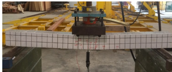
Figure 8. Crack patterns of control beam.
