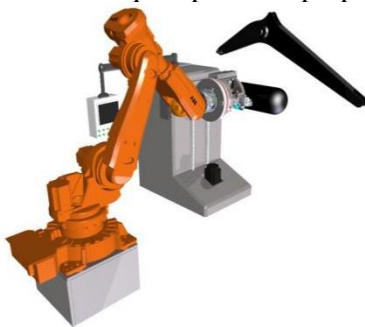
Figure 1: Filament winding robot prototype [9] Figure 2: Filament winding process schematic [10]
