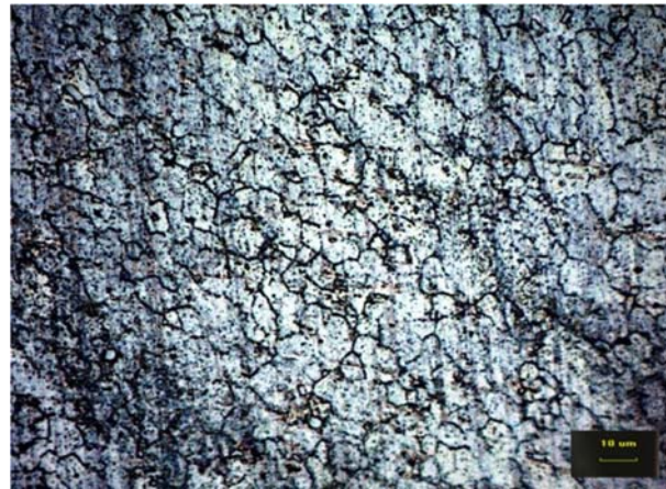
Figure-1. Microstructure of Stir zone for groove size of 3 mm×1 mm.
