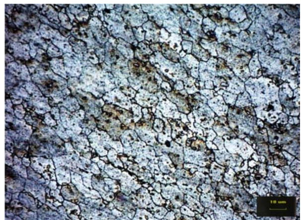
Figure-2. Microstructure of Stir zone for groove size of 3 mm×2 mm.
