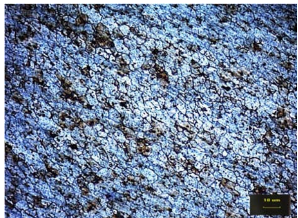
Figure-3. Microstructure of Stir zone for groove size of 2 mm×1mm.
