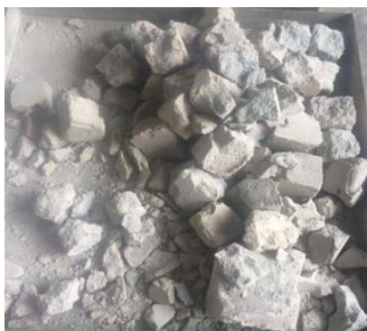
Figure 1. Foamed concrete block chunks.
