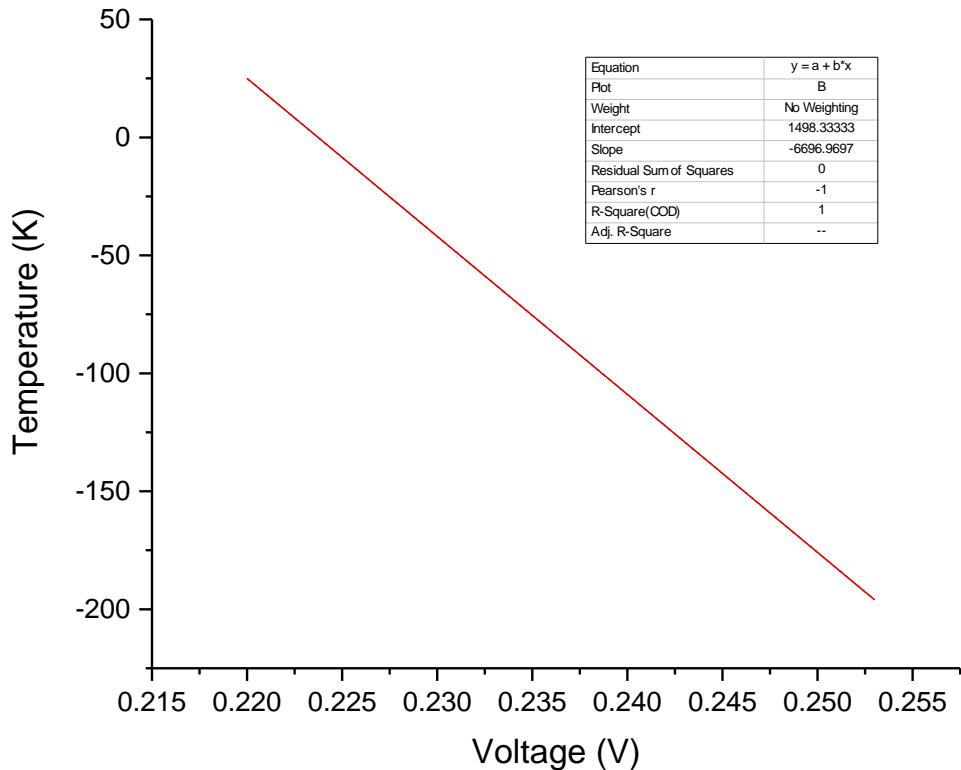
Using the function of the line  $y = -6696.97x + 1498.33$ , the corresponding recorded temperature of the thermocouple was calculated.
