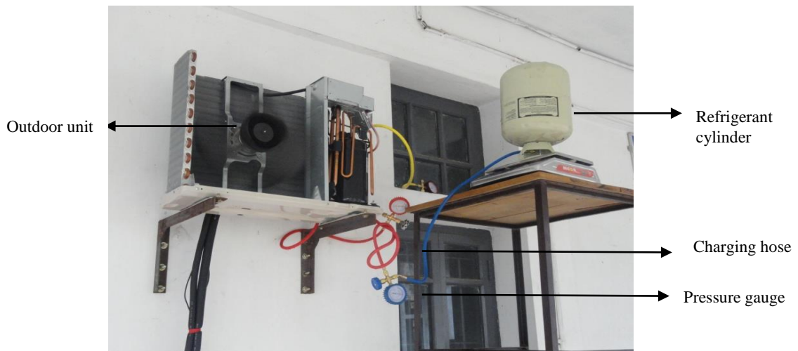
Figure 2. Experimental setup in laboratory and refrigerant charging system.
