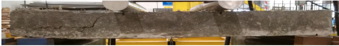
Figure 10. Cracking pattern at the failure of S1-2.
