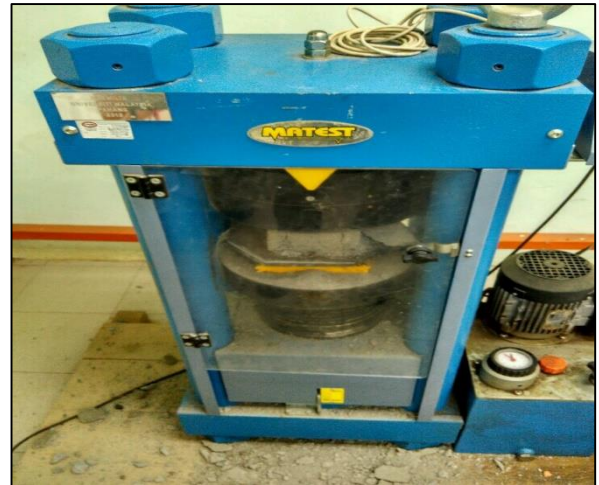
Figure 7: Compressive strength test in progress
