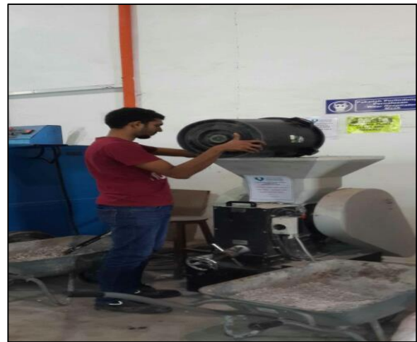
Figure 2: Palm oil clinker pulverizing process
