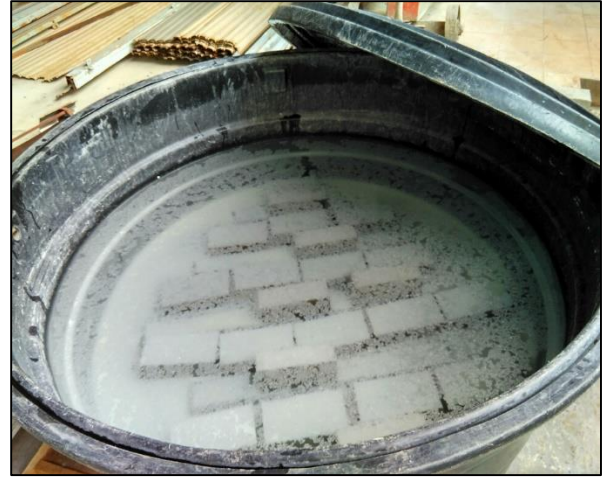
Figure 6: Specimen subjected to water curing
