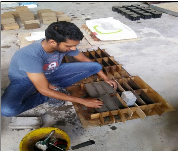
Figure 5: Casting of brick specimen
