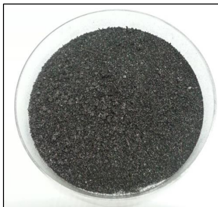
Figure 1. MGSC_{aps} was successfully synthesised using arenga palm sugar as carbon source
