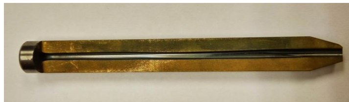
Figure 2. The sectioned nozzle and the silicon casting of WC.
