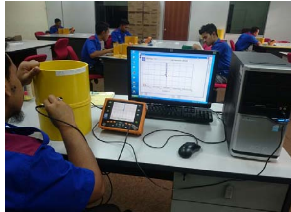
Figure-6. Experimental setup for carbon steel pipe weld coating defect inspection using eddy current testing.
