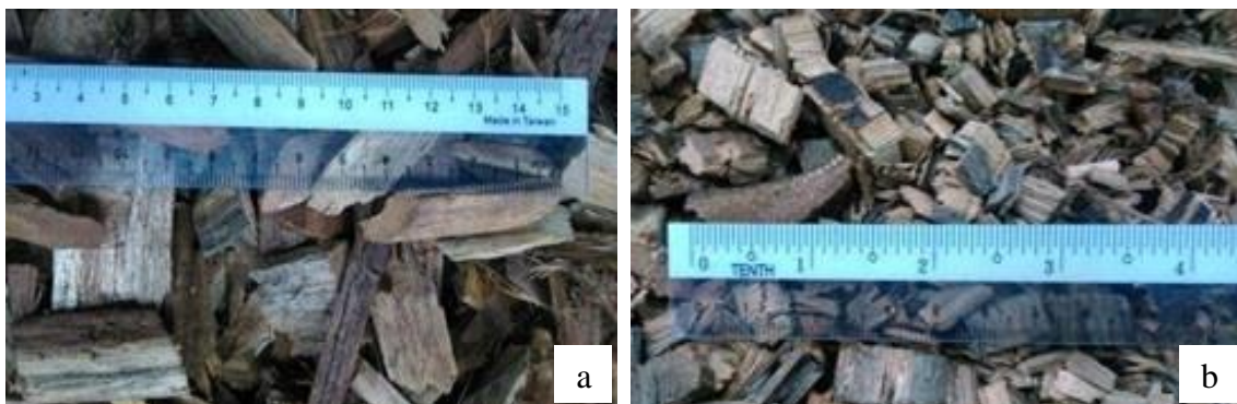
Figure 1. Prepared feedstock of (a) wood chips and (b) coconut fronds for co-gasification.
