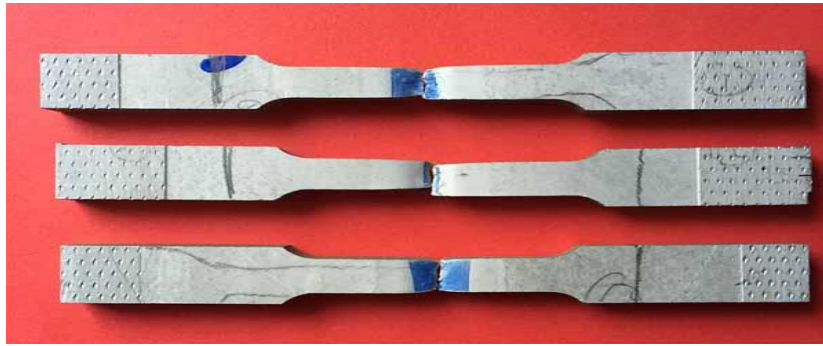
Figure 3: Fractured Tensile specimens at 1200rpm
