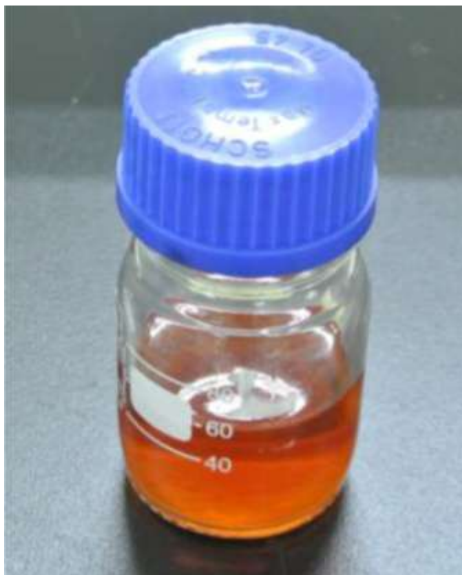
Figure 3. 1: Shellac solution in THF solvent
