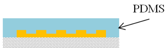
Figure 8. Mixture of PDMS on SU-8 mould.
