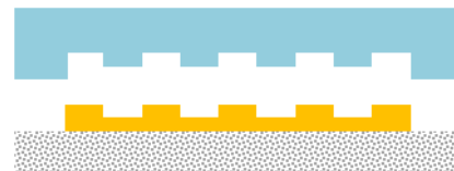
Figure 9. PDMS mould was removed from SU-8 mould.
