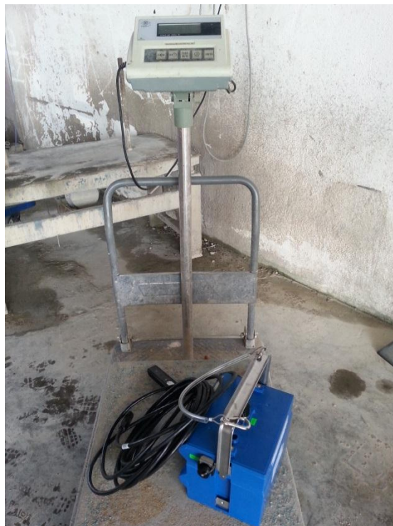
Figure 3.2: Weighting flowmeter (including batteries and sensor)
