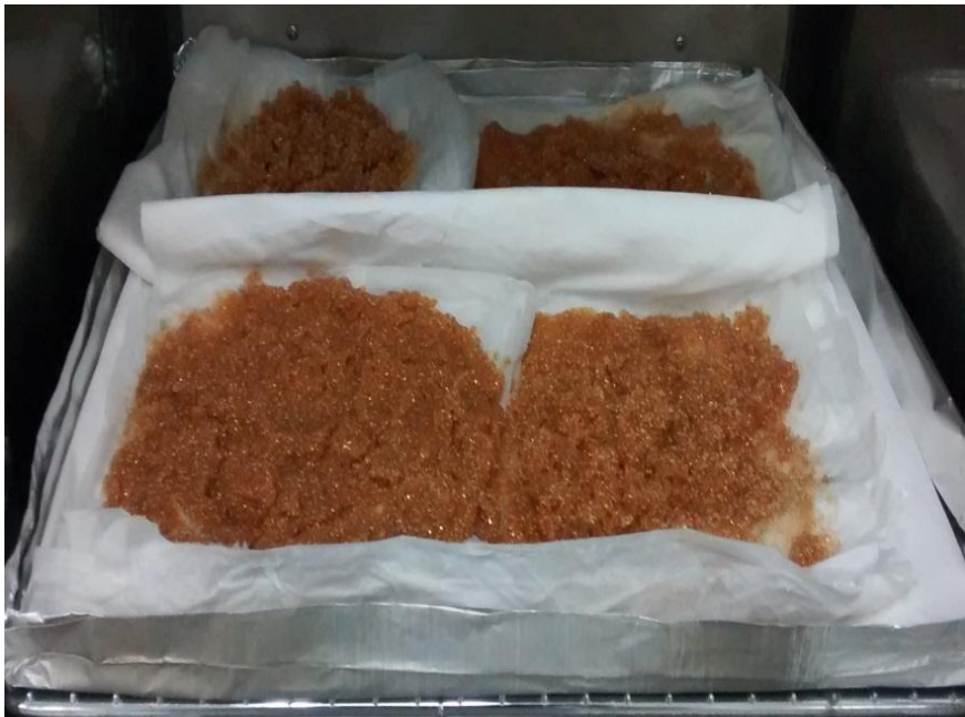
Figure 3-1: Drying of Amberlite IR120 resin.
