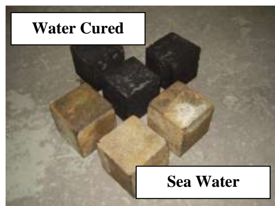
Figure 2 : 1 year water cured POFA cubes with sea water cured specimens
