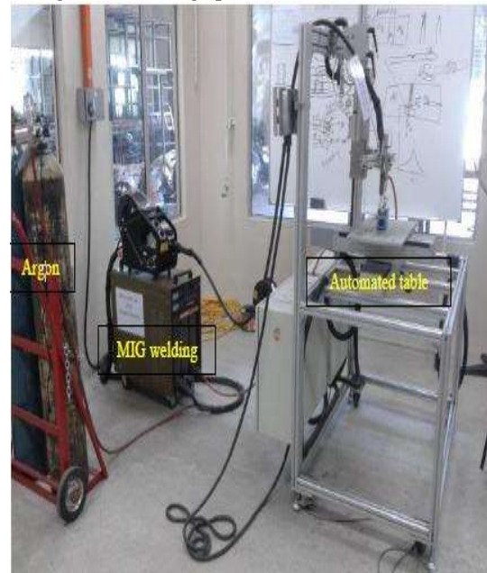
Fig. 1. Automated table and MIG welding type Dr Well DM-500
