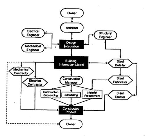
Figure 2.1: The concept of BIM
