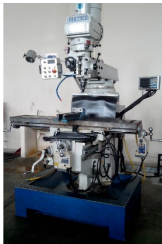
Figure 2. Milling machine (VMM3917 Partner).
