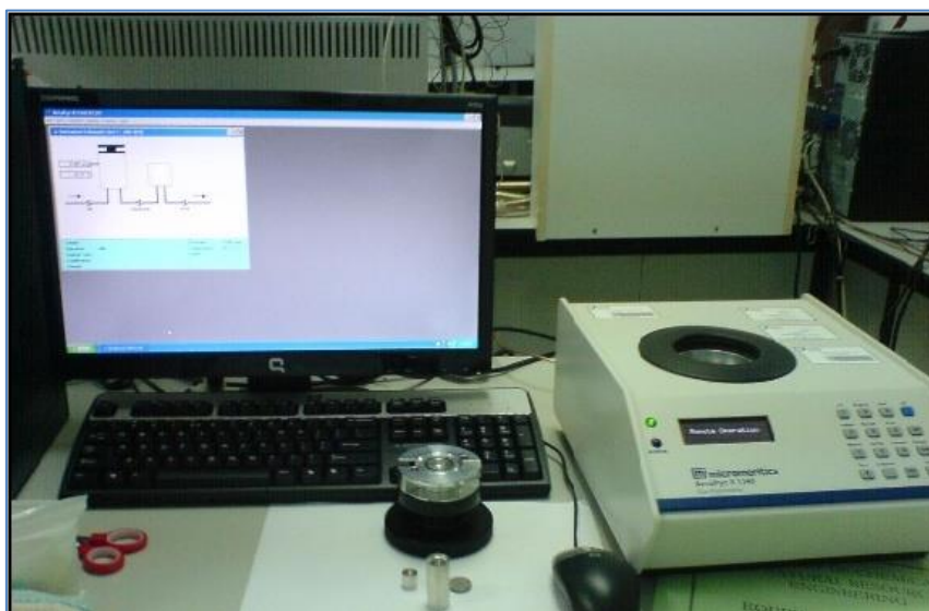
Figure 3-10 Helium gas displacement Pycnometer type 1305 Micromeritics
