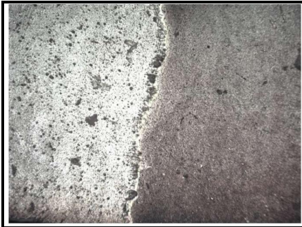
Fig 4 Microstructure of weld interface at 100x
