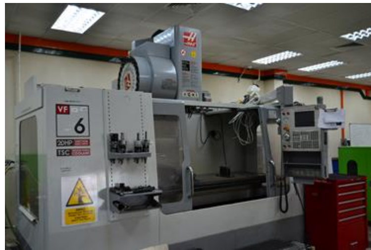
Figure 1. CNC end milling machine HAAS VF-6
