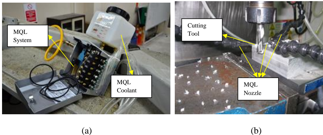
Figure 2. (a) MQL system and UNIST 2210 coolant; (b) configuration of nozzles
