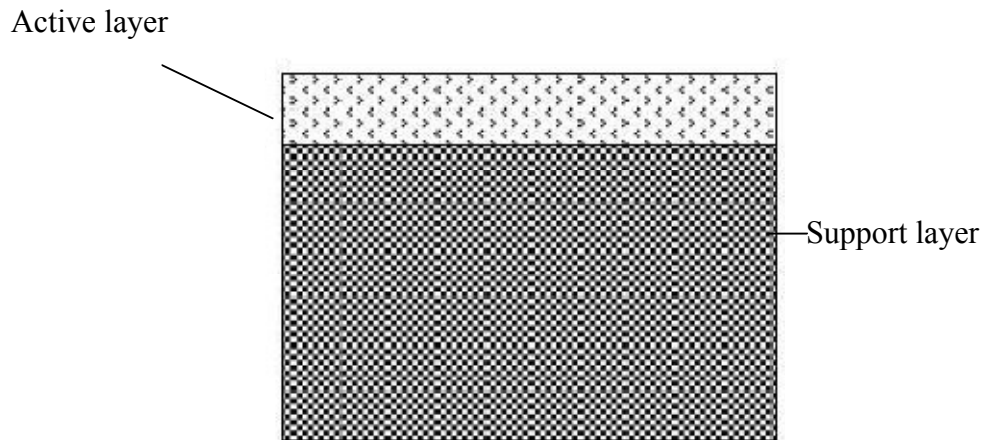
Figure 2.4: Schematic Illustration of Thin Film Composite Membrane
