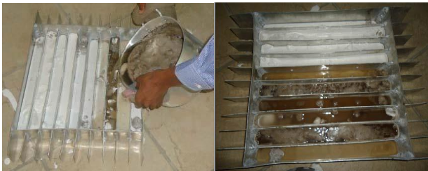
Figure 10. PCMs melted and pouring.
