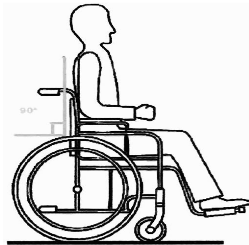
Figure 2.2: Seating position of manual wheelchair
