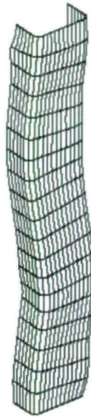
Figure 4.25: Failure mode of SHS 60×60×5 stub column FE model
