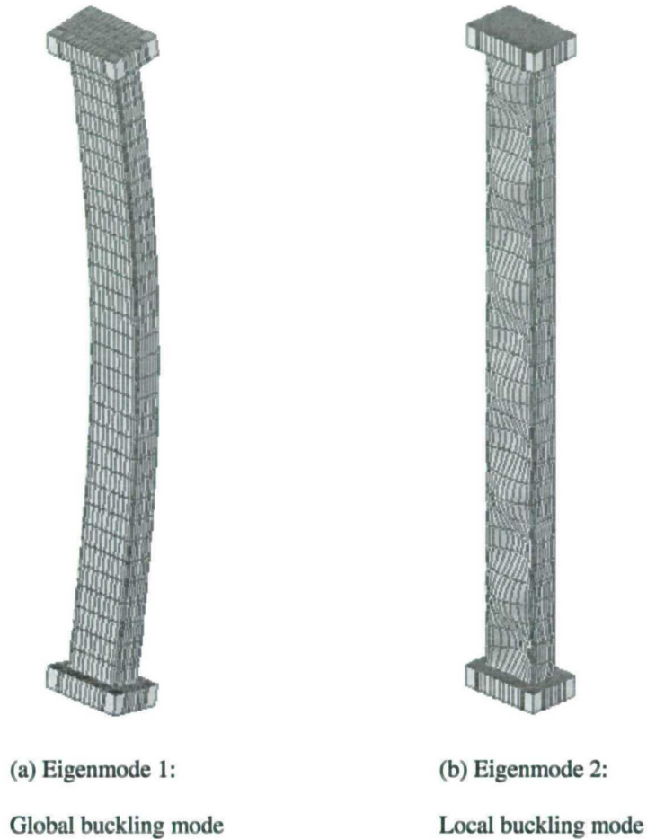
Figure 4.30: Two lowest eigenmodes for 1m pin-ended RHS 100×50×3
