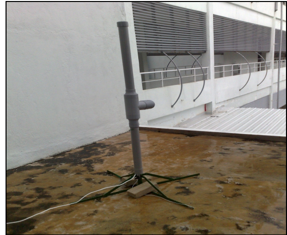
Figure 2. Wire Antenna to detect EF signals
