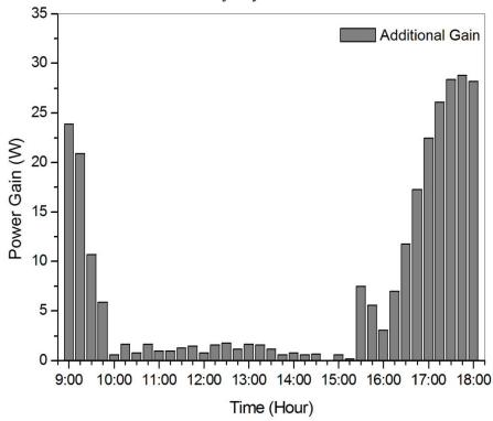
Figure 8. Additional power gain from single-axis tracking solar panel on a partly cloudy day
