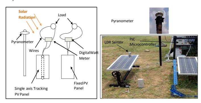
Figure 1. Schematic diagram and actual photograph of PV Solar Panels
