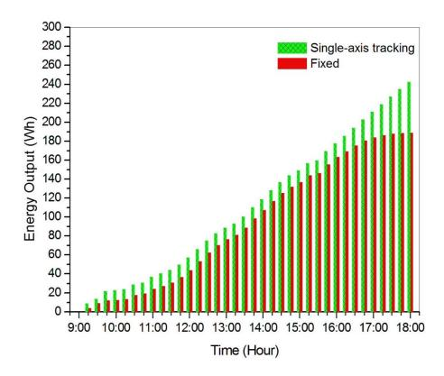
Figure 9. Total energy output from single-axis tracking and fixed solar panel on a clear sky day
