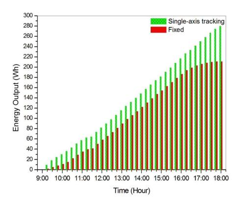
Figure 6. Total energy output from single-axis tracking and fixed solar panel on a clear sky day
