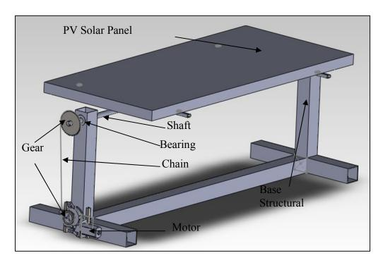
Figure 2. CAD drawing of Single-axis tracking PV
