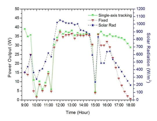
Figure 7. Power output comparison between single-axis tracking and fixed solar panel on a partly cloudy day
