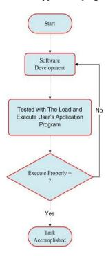
Fig. 3. Monitor Program Testing
