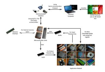
Fig. 1. Block diagram of UMP-EVT
