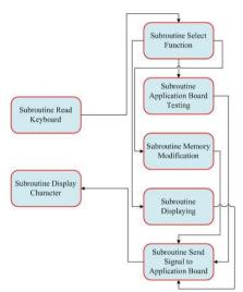
Fig. 2. Concept Diagram of Monitor Software
