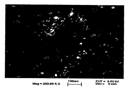
Figure 2.1: Dried alumina nanoparticles
