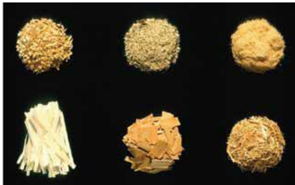
Figure 2.1(a): Common Wood Elements used in Wood based Composites
