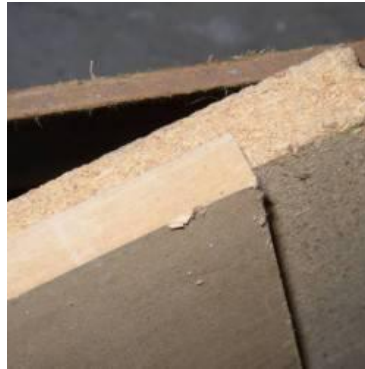
Figure 2.2(b): Wood Fibreboard after Pressing
