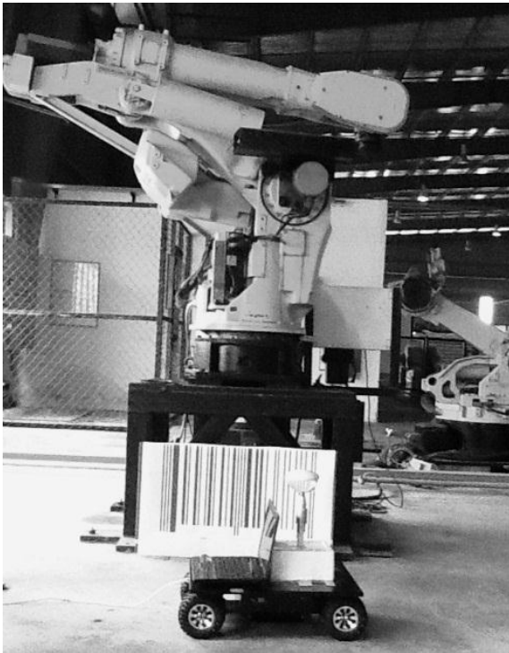
Figure 3: AGV reading barcode in mock manufacturing floor
