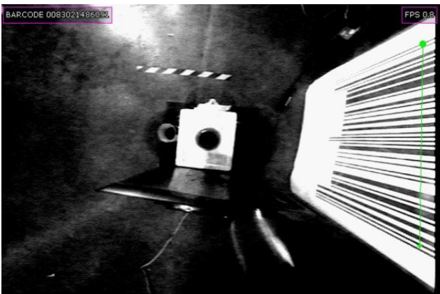
Figure 1: Barcode detection on distorted image.
