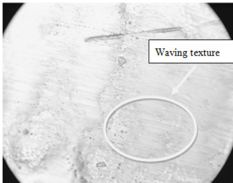
Figure 7. Microscope picture for roughness at condition material thickness 6 mm, tip distance 9.5 mm, cutting speed 2600 pulse/s and power 92.5%.
