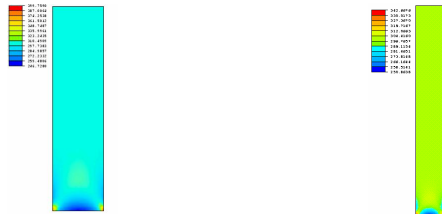
(a) 80mm X 20mm (b) 80mm X 10mm FIGURE 7: Stress distribution by simulation
