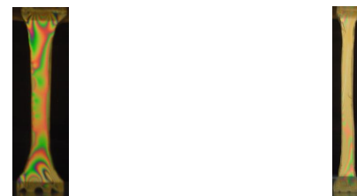
(a) 80mm X 20mm (b) 80mm X 10mm FIGURE 11 Stress distribution for optimum plate.
