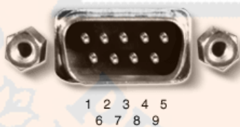
Gambar 2.5 Port serial male (DB9)
