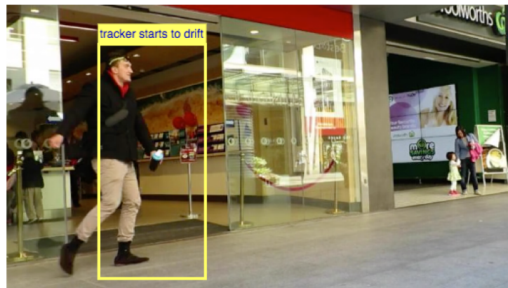
Figure 3.4: The target’s auxiliary template may be updated with wrong image content when a tracker starts to drift since much background information is included within the tracker’s bounding box.
