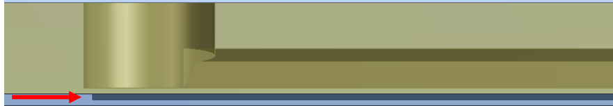
Figure 60: Detail of inlet/outlet path and weld zone aluminum-copper in bottom.
