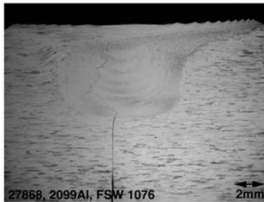
Figure 19: JLR imperfection in FSW.
