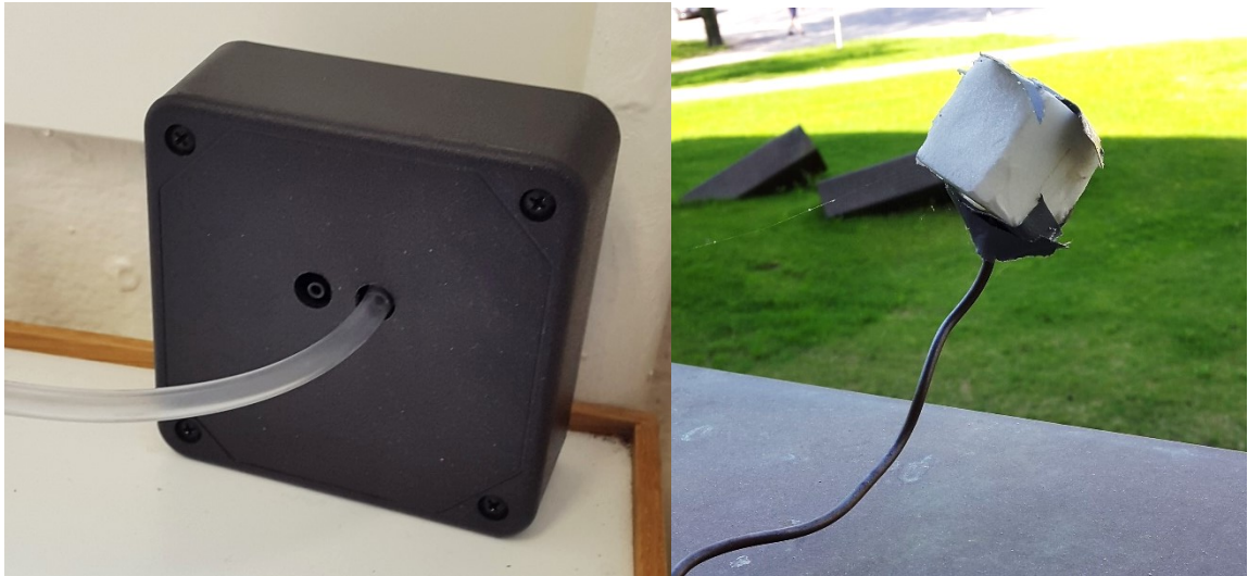
Figure 23. On the left the pressure sensor and on the right outdoor pipe of the pressure sensor with extruded polystyrene placed on top.
