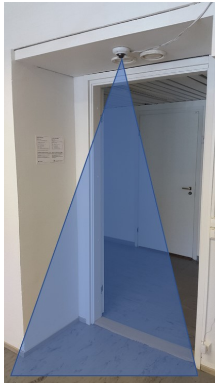
Figure 26. Measurement setup for the AXIS M3045-WV sensor.
