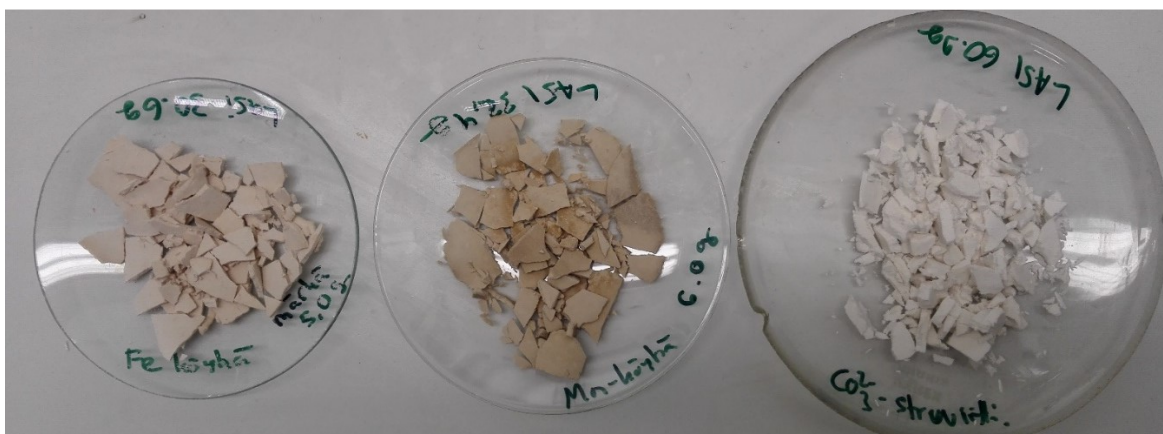
Struvite products after drying in 45°C in VWR Dry-line oven for 16.5 hours. On the left, struvite produced from Fe-poor solution, struvite produced from Mn-hydroxide solution in the middle and on the right, struvite produced from Mn-carbonate solution.
