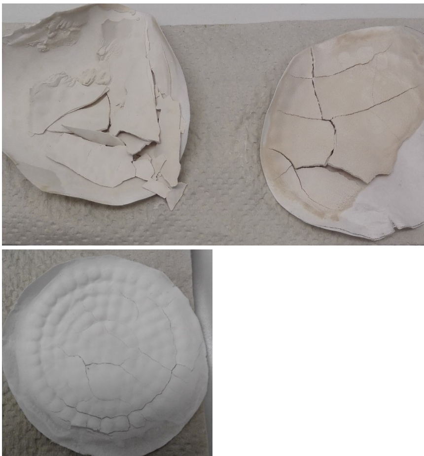
Struvite products after being on the table of the laboratory overnight. On the left, struvite produced from Fe-poor solution, struvite produced from Mn-hydroxide solution in the middle and on the right, struvite produced from Mn-carbonate solution.
