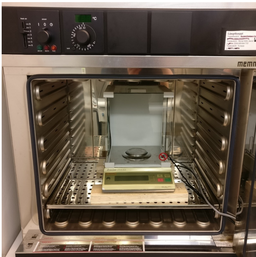
Figure 6. The setup used to measure the weight change (loss of water) in drying CNC suspensions, against time. The samples were placed, one at a time, inside the scale, which collected data during the course of evaporation. The oven door was closed during the experiment.
